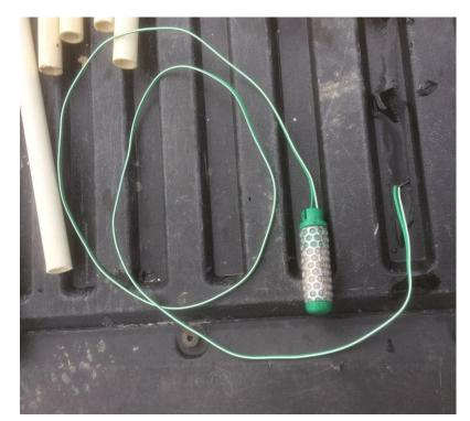
The moisture probe works by measuring electrical resistance in the soil, mimicking the ease or difficulty a plant root has accessing water in the soil. If the soil is wet, electrical conductivity is high, *reducing* the resistance and giving a low reading (below 20 kPa). When the soil is dry, electrical conductivity is low, *increasing* resistance and producing a high reading (above 20, ideally not higher than 60 kPa).
